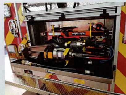
Rear B-1 compartment ideal for hydraulic rescue tools or booster reel
