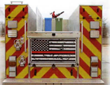
Large hosebed with enclosed ladder and hard suction storage
