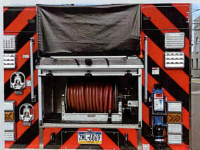
Rear B-1 compartment ideal for hydraulic rescue tools or booster reel
