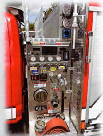
24" wide module affords easy operation and accessibility. Low double-stack crosslays
